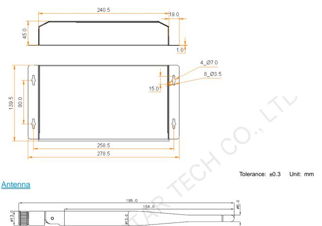
Tolerance: ±0.3 Unit: mm
