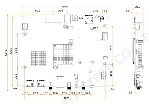
Tolerance: ±0.3 Unit: mm
