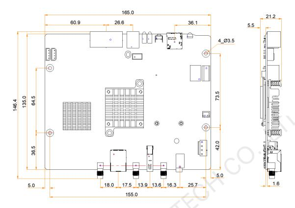
Tolerance: ±0.3 Unit: mm
